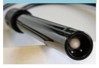
Measuring cell LF 209, 2 pole titanium: nearly maintenance free, applicable up to 5000 µS/cm.
