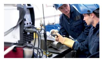
In many industrial processes temperature is one of the most important parameters. For example, measuring the surface temperature within split seconds before the welding process. Fast surface measurements on metal surfaces are the strength of the G 120x and its matching surface probes.
