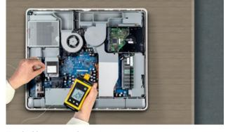
**Heat build-up test on electronic components:** An indispensable aid for troubleshooting of electronic development and electrical equipment services. In addition, the simple and inexpensive GTF 300 wire probe can be used for a wide range of measurements.
