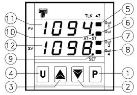
1 - Key P : This is used to access the programming parameters and to confirm selection.
