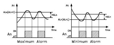
For the band alarms, the example of the low alarm is applicable to the low threshold ("ALnL") while the example of the high alarm is applicable to the high threshold ("ALnH").
