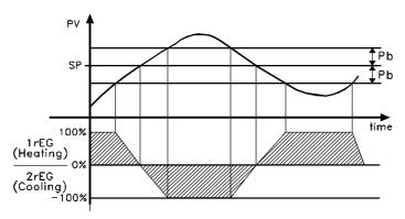
**note** : In order to simplify the explanation of the example graphs a dual action control that is only proportional (and therefore with "dEr" and "Int" = OFF) with "Prat" = 1.0 and "rS" = 0.0 was considered.
