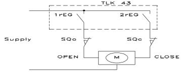
The PID control algorithm for motorised actuators with time positioning foresees the setting of the following parameters: "**Pb**" - Proportional band
