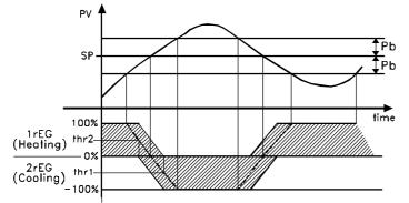
The split range function is deactivated by setting the respective parameters =0.
