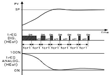
In order to obtain good stability of the process variable, in the event of fast processes and with control by digital output, the cycle time "tcr1" has to have a low value with a very frequent intervention of the control output.
