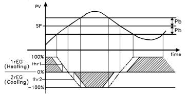
Vice versa if one wishes to extend the reverse action (1rEG) and bring forward the direct action (2rEG) it is necessary to set negative values on parameter "thr1" and positive values on parameter "thr2".
