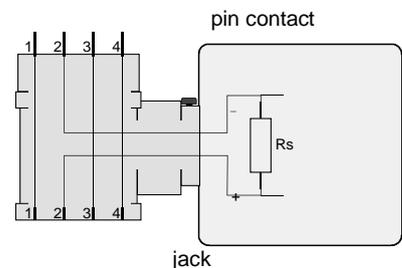
If the 'signal/GND'-line in your transmitter is not assigned to contact 2, please do not forget to adjust the logger-angle-type plug and the external angle-type plug accordingly:
