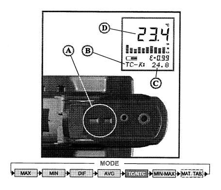
Connect the probe to the input (A). Press MODE, until the desired probe symbol (B) appears. The probe temperature is shown in the lower part of the display (C). The real time infrared temperature is shown in the main display (D).
