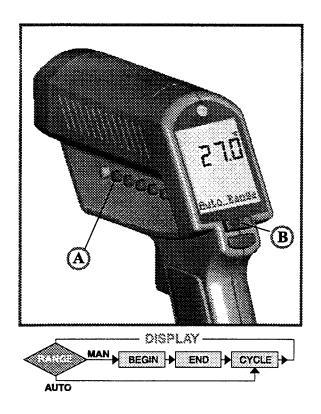
Press DISPLAY (A) once. Use the Up and Down keys (B) to toggle between ranges. Auto Range is automatically defined by the measured maximum and minimum value. Manual Range (Man Range) is user defined (see DISPLAY BEGIN section).
