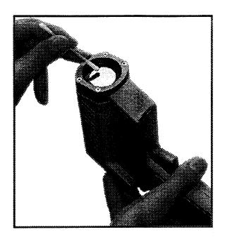
Lens Cleaning: Blow off loose particles using clean compressed air. Brush remaining debris away with a camel's hair brush. Wipe the surface with a moist cotton swab. The swab may be moistened with water or a water based glass cleaner. NOTE: DO NOT use solvents to clean the plastic lens.
