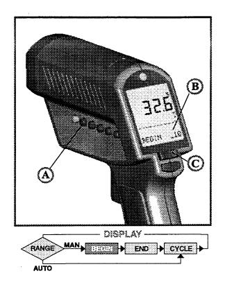
To set the BEGIN value for the graphic display (Man Range is activated) press DISPLAY (A) until "Begin" is shown at the status bar. Use the Up and Down keys (C) to select the value (B).
