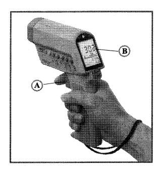
To take a temperature measurement, hold the unit as shown. Aim at the target. Pull the trigger (A). The temperature of the object being measured is shown on the display (B). The temperature will be displayed for seven seconds after the trigger is released.
