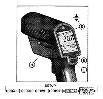
This function is used with a selected emissivity to add or subtract an offset value  $(\pm 10^{\circ}\text{C}/\pm 18^{\circ}\text{F})$  to the temperature value. This allows several units or a specific temperature range to be matched. Press the Setup button (A) until "Offset" appears in the display. With the arrow keys (B) choose the value. Press enter (C) to confirm. If offset is used, a symbol (D) appears in the display.
