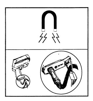
Keep away from EMF (electromagnetic fields). Avoid static electricity, arc welders, induction heaters. Don't leave the unit on or near objects of high temperature. WARNING: DO NOT touch live voltage with contact probe. Use the wrist strap for cable support.
