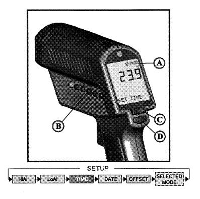
To set time, press SETUP (B) three times. Change the time (A) using the Up and Down keys (C). Then press ENTER (D) for each time segment to activate this time setting. The time appears on the display, is stored within the data logger and is part of the printer output.
