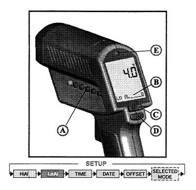
The low alarm (LoAl) generates an audible and visual (flashing LED and laser) (E) alarm if the temperature is below the setpoint.
