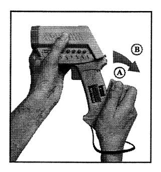
To open the battery compartment, press gently on the top part of the handle (A) to release the catch (B) and pivot the grip as shown in the figure. Orient the batteries (two alkaline R6 (AA, UM3)) as shown on the housing.
