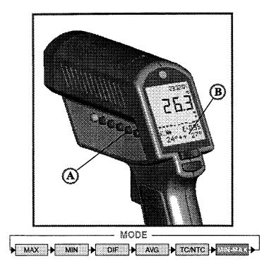
To show the minimum and maximum temperature values during a measurement at the bottom of the display, press MODE (A) until the two values appear (B).
