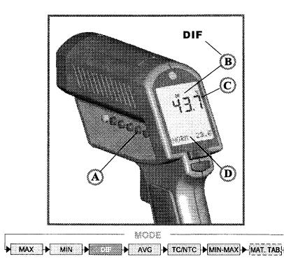
To activate the DIF mode, press MODE (A) until the DIF symbol (B) appears. The difference between the measured max and min temperatures is displayed (C) as long as the trigger is pulled or locked on. The real-time temperature is shown in the lower part of the display (NORM) (D).
