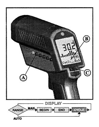
CYCLE allows the adjustment of the display interval. Press DISPLAY (A) until Cycl.: (B) is shown at the status bar. To select the interval time, use the Up and Down keys (C). The default value is pre-set for 0.5 sec.
