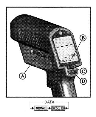
To store data, press DATA (A) once. "RCL" will flash and a log location will be shown at the status bar (B). To select another log location, use the Up and Down keys (C). Press ENTER (D). "LOG" will be shown. Pull the trigger, release again. Store by pressing ENTER (D). You will hear a tone. To exit, press DATA once.
