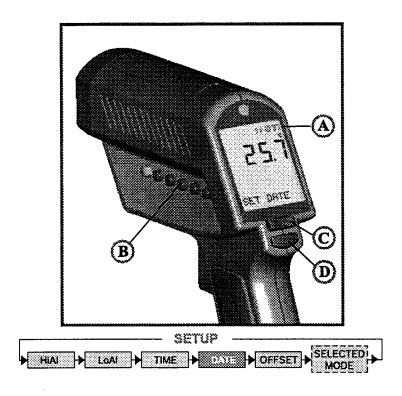
To set date, press SETUP (B) four times. Change the date using the Up and Down keys (C). Then press ENTER (D) for each date segment to activate this date setting. The date (A) is stored within the data logger and is part of the printer output.
