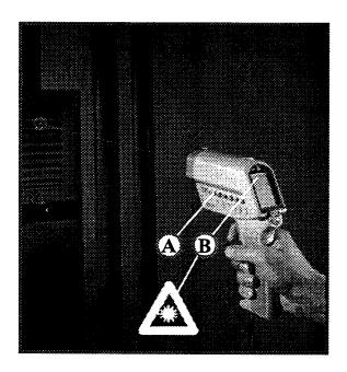
The laser circle shows the spot size that includes the measured target. To turn the laser on or off press the LASER button (A) when the trigger is pulled. A laser symbol (B) appears when the laser is on. The laser automatically turns off if you release the trigger.
