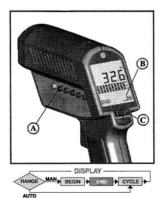
To set the END value of the graphic display (Man. Range) press DISPLAY (A) until "End" is shown at the status bar. Use the Up and Down keys (C) to select the value (B).
