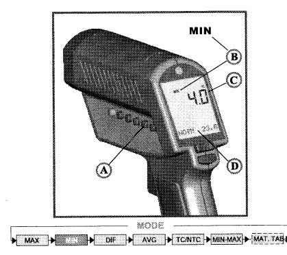
To activate the MIN mode, press MODE (A) until the MIN symbol (B) appears. The measured minimum temperature (C) is displayed as long as the trigger is pulled or locked on. The real time temperature is shown in the lower part of the display (NORM) (D).
