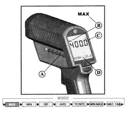
To activate the MAX mode, press MODE (A) until the MAX symbol appears (B). The measured maximum temperature is displayed (C) as long as the trigger is pulled or locked on. The real time temperature is shown in the lower part of the display (NORM) (D).
