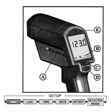
The high alarm (HiAl) generates an audible and visual (flashing LED and laser) (E) alarm if the temperature is above the setpoint.
