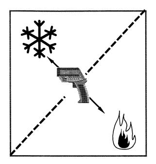
Avoid abrupt changes in temperature. If this occurs, allow 40 minutes for thermal stabilization before use to prevent the possibility of inaccurate temperature readings. Please use only the Power Supply from the manufacturer.
