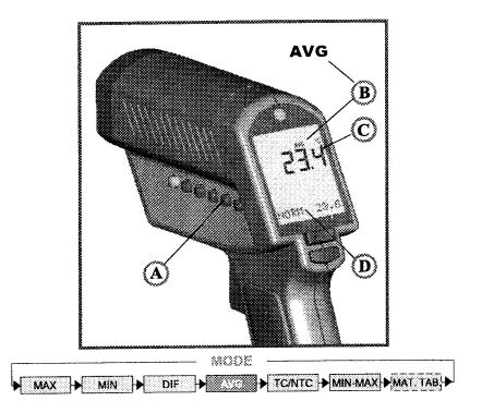
To activate the AVG mode, press MODE (A) until the AVG symbol (B) appears. The average value of measured temperatures (C) is displayed as long as the trigger is pulled or locked on. The real time temperature is shown in the lower part of the display (NORM)(D).
