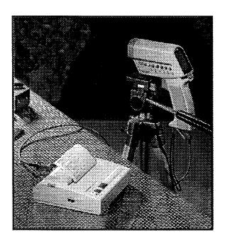
Open battery compartment and switch LOCK "on" to lock the unit on. You may mount the unit on a tripod, utilizing the tripod mount. Pull the trigger for continuous temperature measurement. (The laser will not be locked on.) To unlock, switch LOCK "off".
