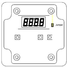
If the jumper is removed from the shown contacts, the configuration is inaccessible, values are protected.
