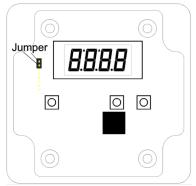
If the jumper is removed from the shown contacts, the configuration is inaccessible, values are protected.
