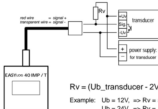
$$R_v = (U_b\_transducer - 2V) / 2 \text{ mA}$$
