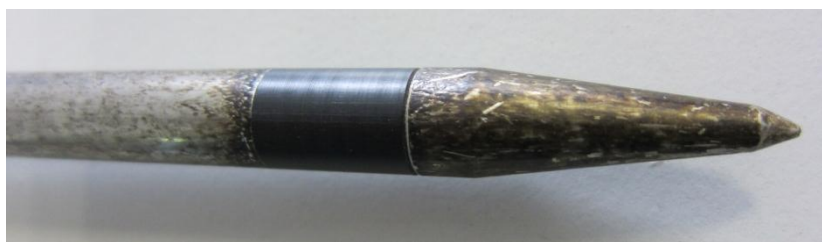
Soiled probe -> wrong measuring!
