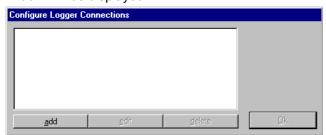
Choose ,add' to add a logger connection to the connection list. There can be added as much connection as needed, the settings can be altered anytime by selecting the desired connection and clicking on ,edit'. A correct setup is necessary for the proper functioning of the software!
