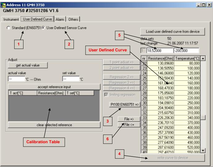
ATTENTION: If the device is equipped with a calibration certificate, the calibration was done by means of the User Defined Sensor Curve. You have to choose (2). If the user changes this curve, the calibration certificate is not valid anymore. If the device is switched to the standard curve, the device does not measure with the calibration data of the certificate!
