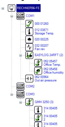
The main settings and adjustments of the program can be done at the Navigation panel. Here the bus system is selected, connected modules are searched for and the device or recording settings are adjusted.
