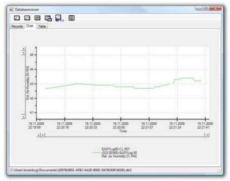
The Y-axis is labelled corresponding to type of measurement and unit. (There will be no axis label, if no valid type or unit exists.)
