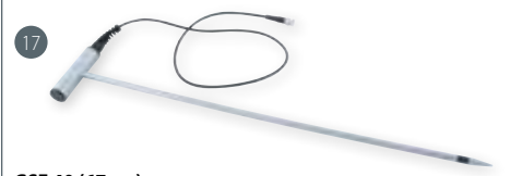
GSF 40 (67 cm) Item No. 601316 Material moisture insertion probe, (without temperature sensor) for measurement in pressed bales at a depth of 60 cm, incl. 1 m connection cable. Suitable for: pressed hay and straw bales, grain
