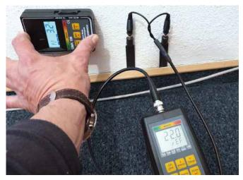
Measurement in screed insulation through edge insulation strips: Moisture beneath screed GMH 3831 with flat electrodes
