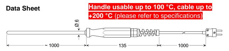
The GTF 1000 AL is an economical sensor for short-term use in aluminum smelters as a cost-effective and break-resistant alternative to expensive and sensitive ceramic sensors.
