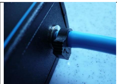
Above 2 bar rel: lock with clamp
