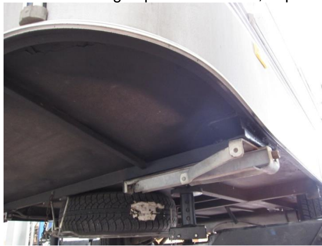
Caravan floor: massive flake board, little protected
