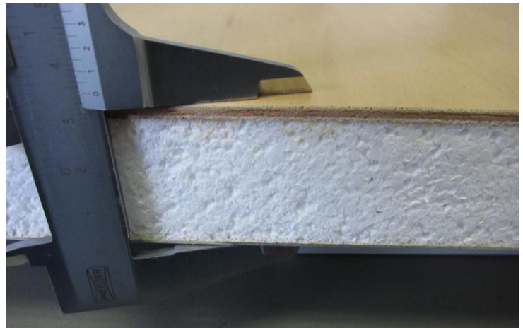
Example sandwich: aluminum - insulation - plywood
