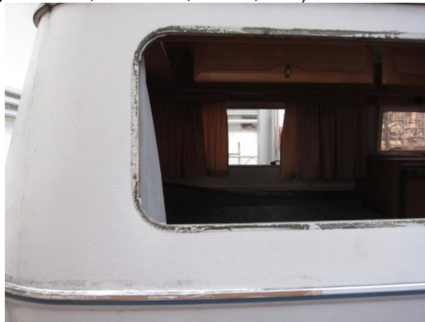
An overview of three possible weak points: roof sealing, window sealing and assembly weld upper to lower trailer body The reason here: old and porous window sealing
