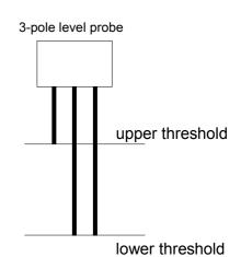
When the fluid-level falls under the MIN-sensor-contact (lower threshold) the power outlet of the controlling device is currentless and therefore the attached device will be turned off. The LED from the controlling device lights.
